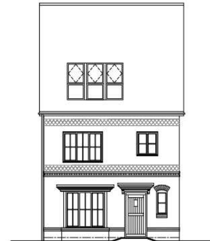
Front Elevation (Tile Hanging)
