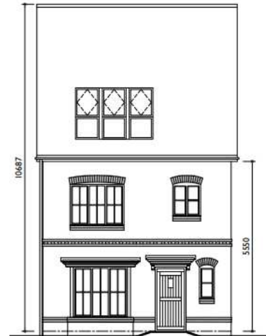
Front Elevation (Brick)
